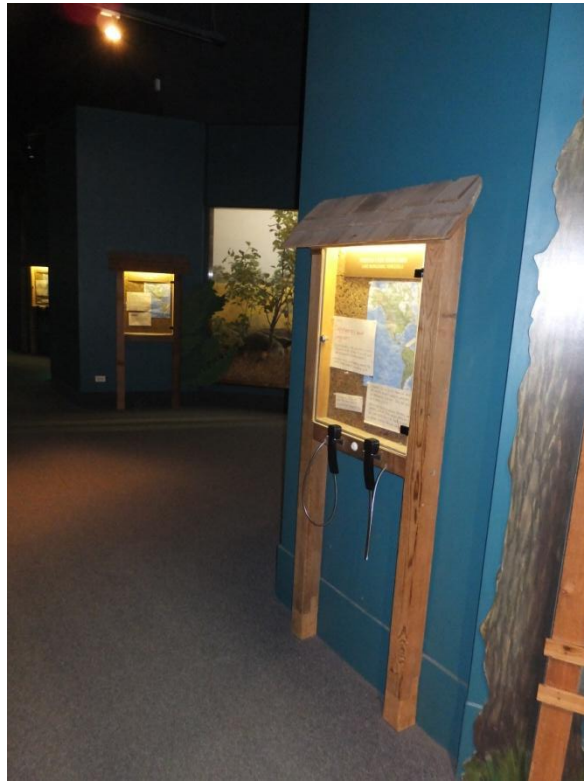
Figure 51 -- The Roof over the Bulletin Board is not Cane Detectable in Message from Wilderness Exhibit
