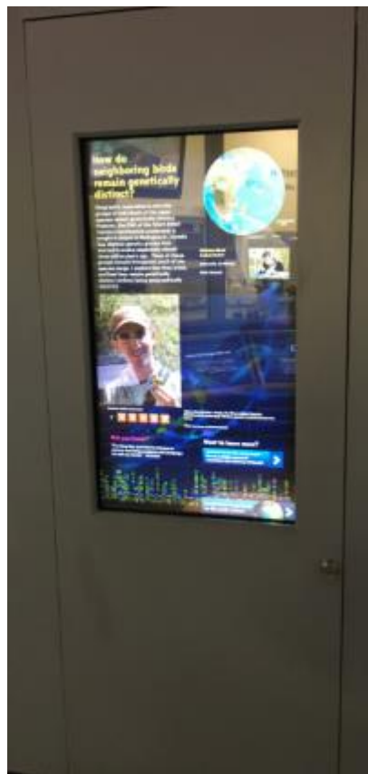
Figure 35: Another example of a digital panel with touch controls too high
